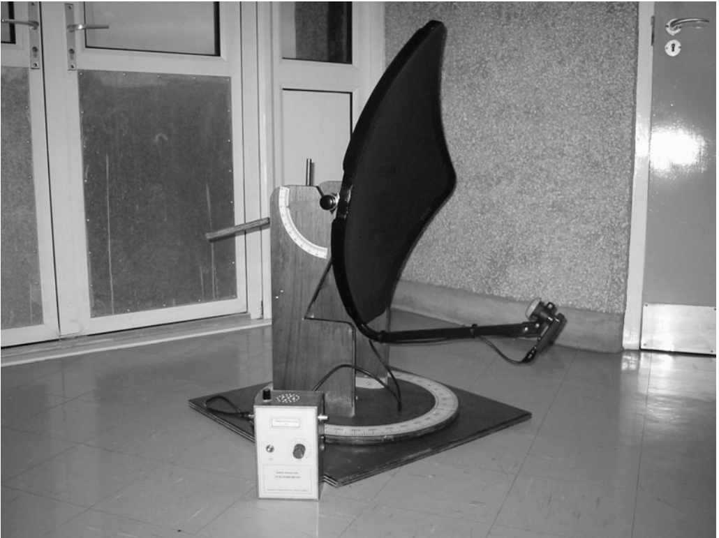
Figure 24.16. A simple satellite receiver dish mounted on an alt-azimuth frame with the output displayed on a power meter.
